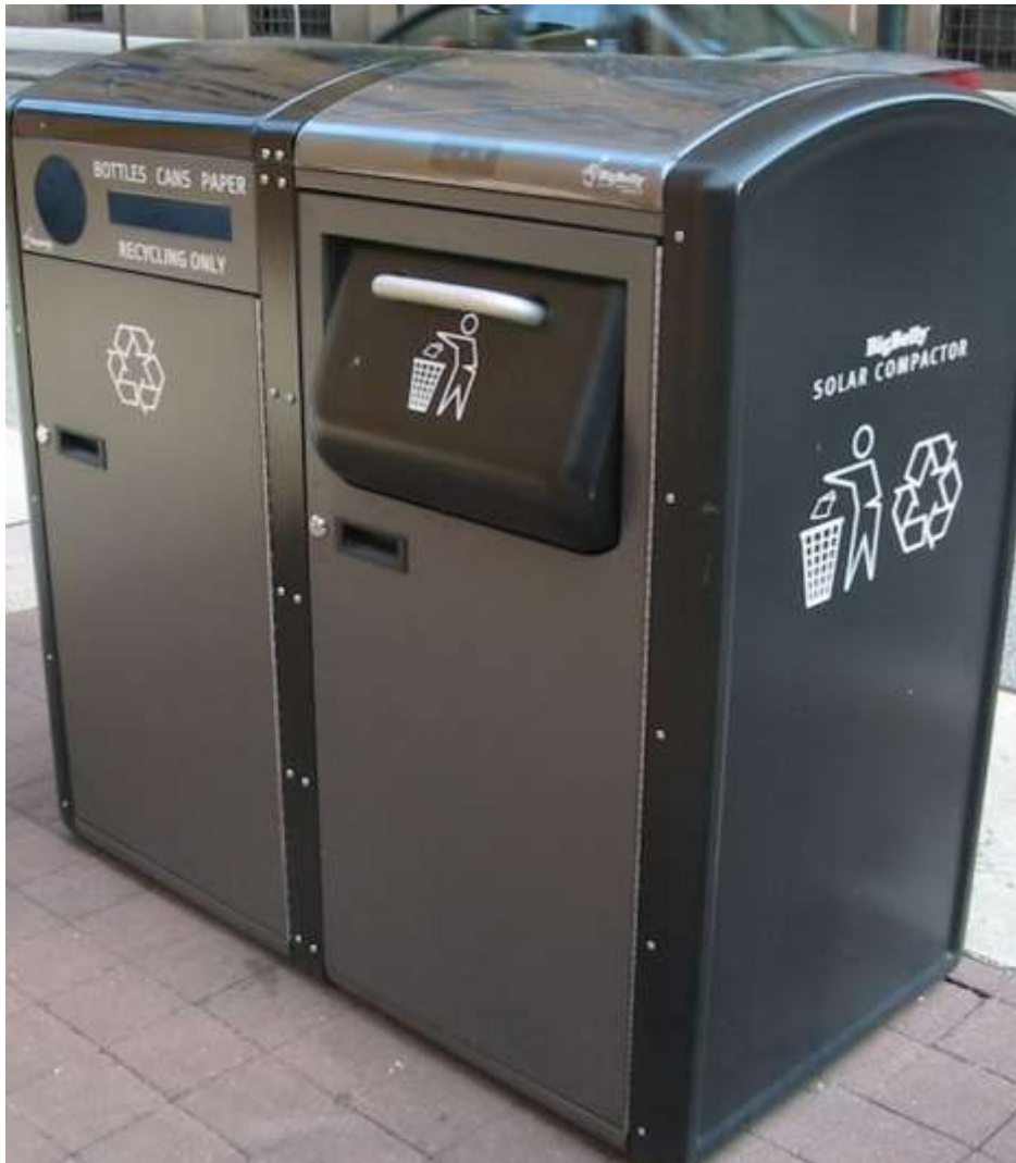
Smart trashcans in New York tell garbage collectors when they need to be emptied. They optimize trash service by ensuring drivers only make necessary stops, and drivers modify their route to reduce fuel consumption.
