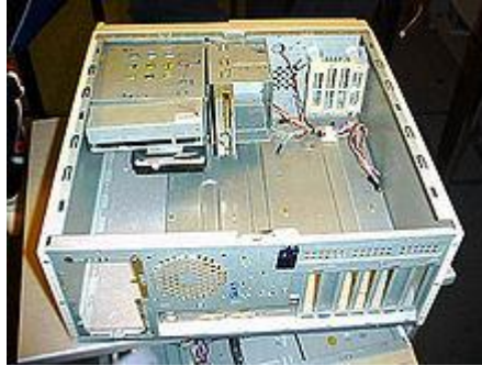
Figure: shows a stripped ATX desktop case. The motherboard will lie flat on the bottom, against the right panel, with peripheral connectors protruding through the rear panel, drive bays at the top and front, and the power supply at the top and rear.
