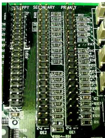
Figure: Left A close-up of the primary and secondary IDE interfaces on a motherboard; Right The connector on an IDE cable, the stripe denotes where to align with Pin 1.
