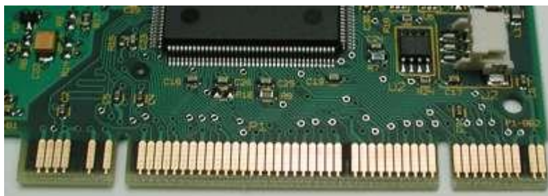
Figure: PCI card showing the pins (4+2+24+10+8+2) and PCI bridge chip.
