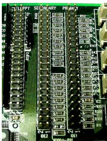
Figure: Left A close-up of the primary and secondary IDE interfaces on a motherboard; Right The connector on an IDE cable, the stripe denotes where to align with Pin 1.
