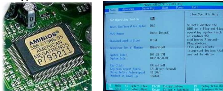
Figure: The BIOS chip and the BIOS setup Utility program
